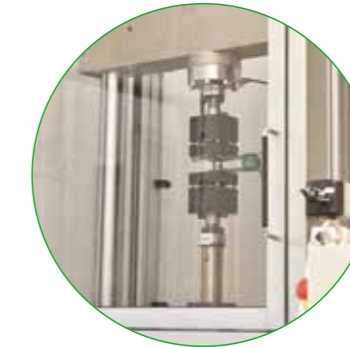
Mechanical testing machine (100Hz Fatigue Test)
